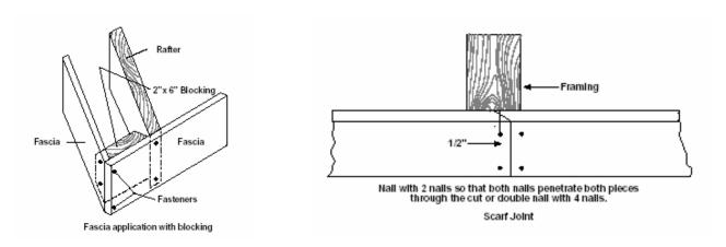
DO NOT USE STAPLES, T-NAILS OR ANY TYPE OF COUNTER-SINKING FASTENER, such as tapered head or bugle head fasteners. Use of these fasteners will void the warranty.
