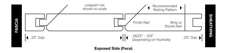
Nails should penetrate framing member at least 1.5" (38.1mm). Screws should penetrate at least 1" (25.4mm). Fasteners should be spaced 24" on center or less. Approved fasteners include: Hot dipped galvanized or aluminum nails = 2.25" (7d) smooth, or 2" (6d) ring shank. 15 gauge brad nails are also approved.
