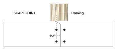
Two nails should penetrate through both boards, otherwise four nails should be used to fasten facsia to framing.
